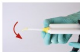
PICTURE 5 Make sure the notches on the Mixing Tip match those on the cartridge. Press firmly to attach the Mixing Tip. Then turn the Mixing Tip 90 degrees in a clockwise direction to its "locked" position. The mixing gun is now ready for use.
