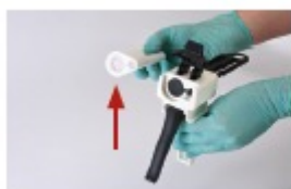
PICTURE 2 and 3 Lift the plastic lever to insert the cartridge. Important: Make sure that the notches on the cartridge match those on the mixing gun. Then lock it by pushing the plastic lever back down.
