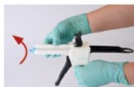
PICTURE 4 To insert the Mixing Tip, remove the cartridge cap by turning the cap counterclockwise 90 degrees, and then pull it off. You can keep the cap to close the cartridge if the contents have not been used up completely.
