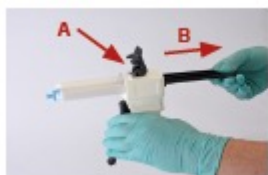
PICTURE 6 and 7 To remove the cartridge, press the mixing gun release lever upwards. (A) Completely retract the lever. (B) Place the cartridge lock in the up position and lift the cartridge out of the dispenser.
