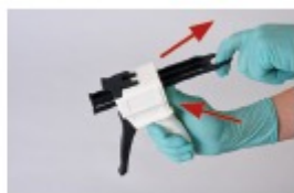
PICTURE 6 and 7 To remove the cartridge, press the mixing gun release lever upwards. (A) Completely retract the lever. (B) Place the cartridge lock in the up position and lift the cartridge out of the dispenser.
