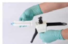
PICTURE 2 and 3 Lift the plastic lever to insert the cartridge. Important: Make sure that the notches on the cartridge match those on the mixing gun. Then lock it by pushing the plastic lever back down.
